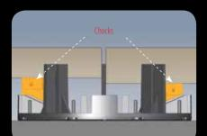
Height Adjustable Allows height adjustments from .95 - 1.77" (24mm to 45mm) in 1mm increments.
